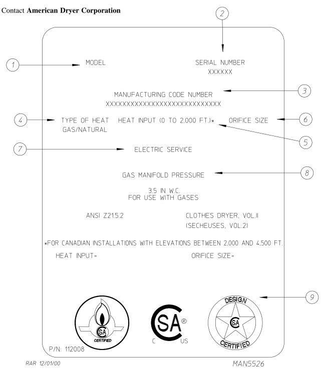
When contacting **American Dryer Corporation**, certain information is required to insure proper service/parts information from **ADC**. This information is on the data label located on the inside of the control door. When contacting **ADC**, please have the **model number** and **serial number** available.
