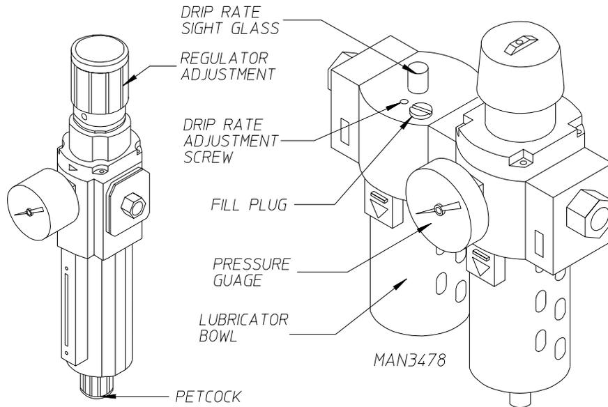
**NOTE: LUBRICATOR *SHOULD BE* SET AT 1 DROP PER CYCLE.**
