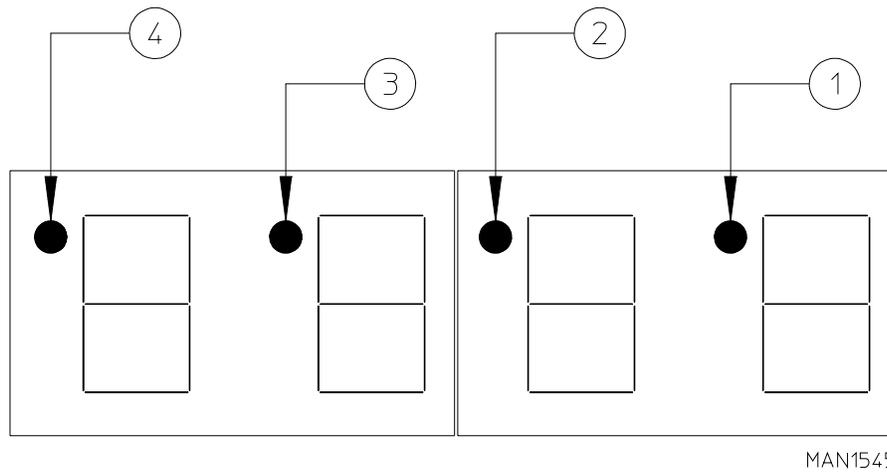
1. Blower Motor Circuit Indicator - indicator dot is on whenever a cycle is in progress.
