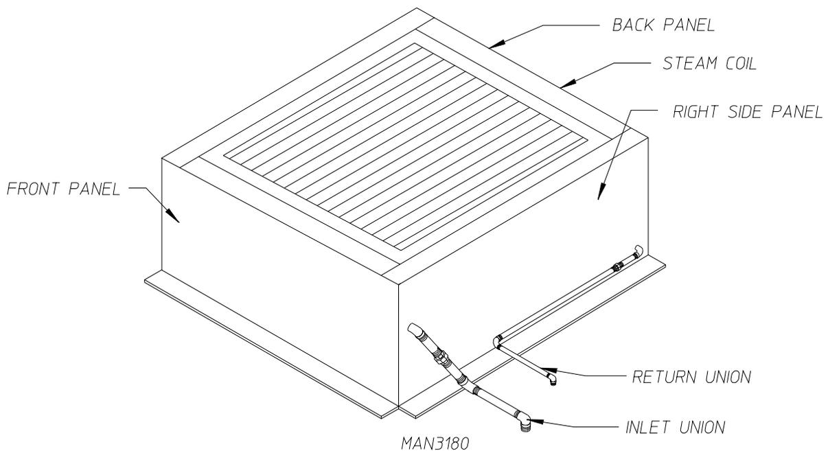
VIEW OF STEAM COIL w/ DAMPER REMOVED
